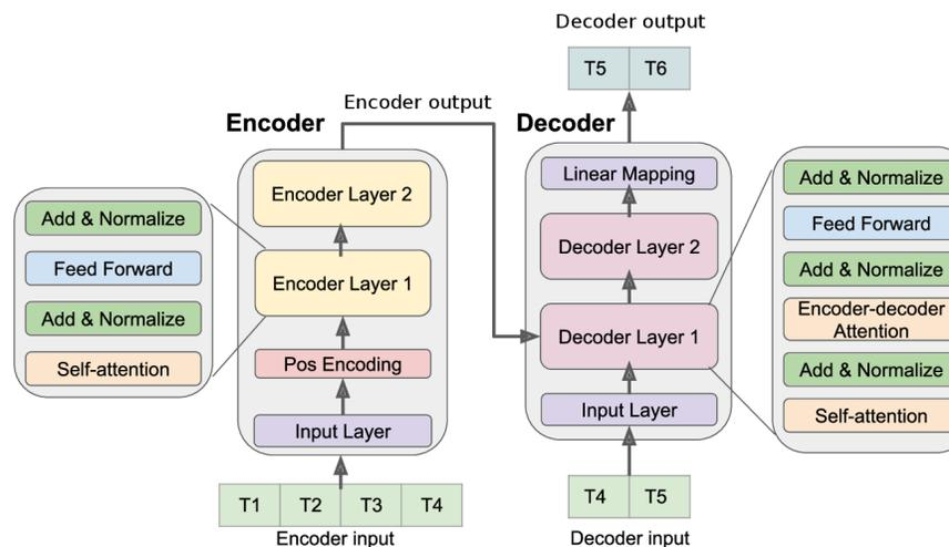
Transformer Models originally designed for NLP
