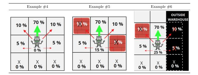
Notice that in example #5, the two locations occupied by a wall prevent the robot from moving into those spaces and therefore the robot stays in place 15% (10% + 5%) of the time. Similarly, any attempt to move outside the warehouse will result in the robot staying in the same location (as seen in example #6).
