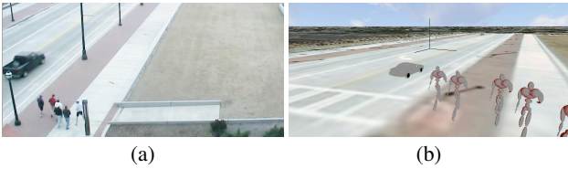
Figure 2: Example of DM: (a)Single video observing pedestrian and car (b)Screen space position mapped onto virtual plane space
