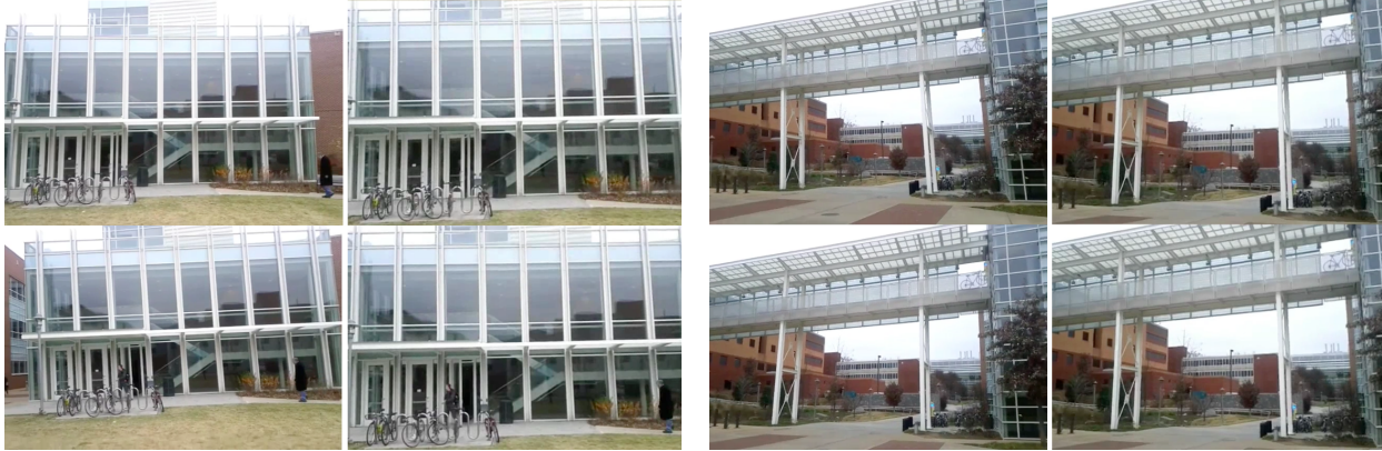
Figure 1: Two examples rectified using our calibration free rolling shutter technique. Original frames on the left, our rectified result on the right. Our model accounts for frame global distortions such as skew (left example) as well as local wobble distortions which compress and stretch different parts of the frame (right example). Please see accompanying video.
