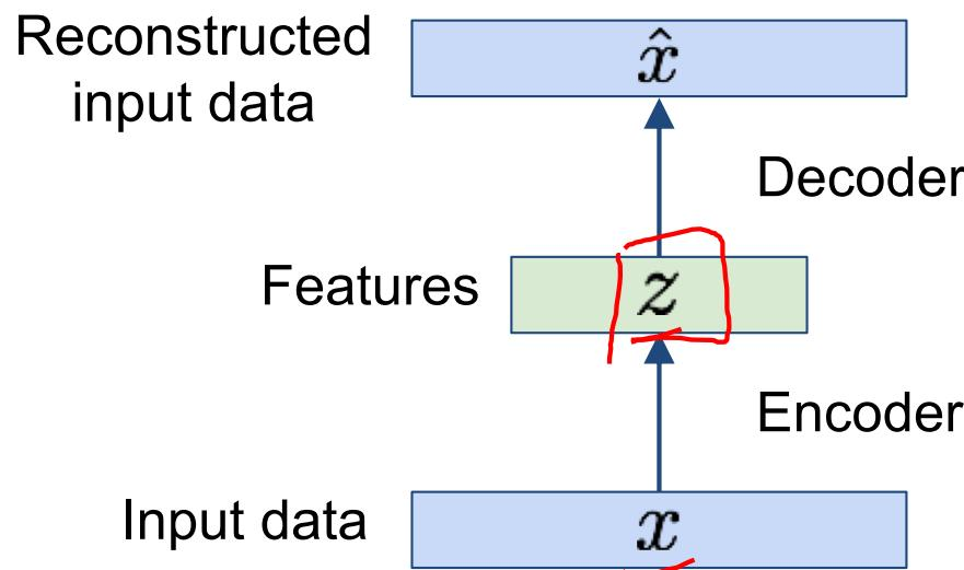
Autoencoders can reconstruct data, and can learn features to initialize a supervised model
