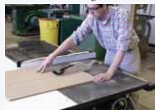
Cut complete. Part between fence and blade must be cleared past blade.
