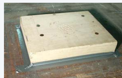
Lift frame and tape box to table. An airtight seal is needed.
