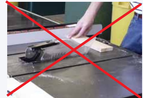
NEVER attempt a crosscut using the fence. Part will Definitely kickback causing injury.
