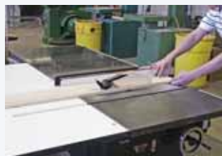
Once part clears table, a Push Stick is used to push pass blade.
