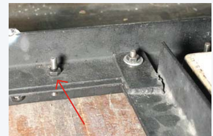
Close up of adjustable frame. Never remove threaded stud and nut. These are for alignment.
