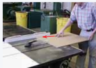
Part held to table. Both hands are applying force toward corner of part.
