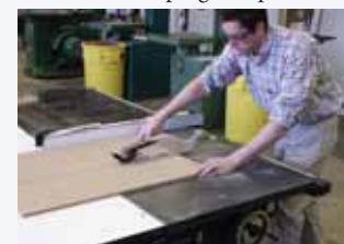
Left hand supports material so it does not pull cut piece into blade.
