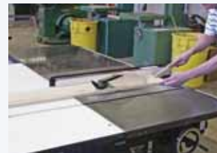
Left hand never pushes part, it supports part against fence.
