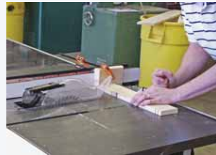
By clamping a stop block to the fence you can make repetitive cuts. This method allows part to fall away and not become lodged and KICKBACK. It would be easier to use other machines.
